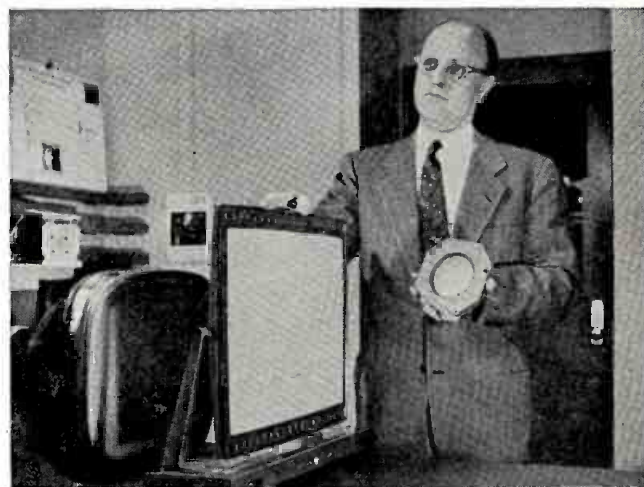
Thin TV set of 1965, as designers imagine it now, is shown next to one of today's TV tubes. Dr. Suits holds in his hand the new light-booster screen developed by Dr. Ferd Williams and D. A. Cusano of General Electric.
